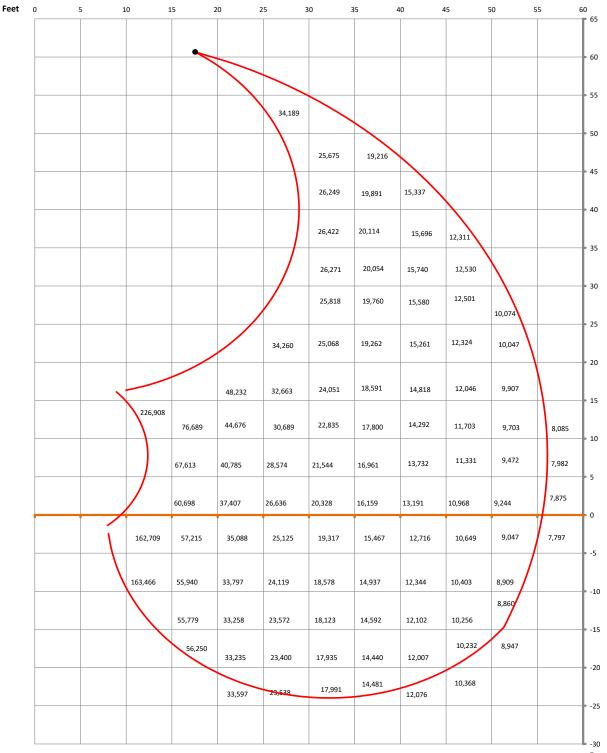
The load capacity number is in unit of pounds and the location is the left upper corner of the box. For example box 34,189 lbs is the load capacity at 25 ft reach and 55 ft height. The reach measurement is from the center point of the rotation bearing to the load point. The height is measured from the load point to ground. The load point is the center line of the attachment pivot mounting pin on the stick.
